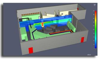
**EPM has developed its own suite of fire modeling tools.** The tools use plant specific information related to ignition sources, combustibles, detection & suppression systems, and targets to calculate severity factors, fire growth analyses, zones of influence, hot gas layer potential, and fire scenario frequency details. For each of these workbooks EPM has completed validation and verification (V&V) reports which document the technical bases for the calculations.
